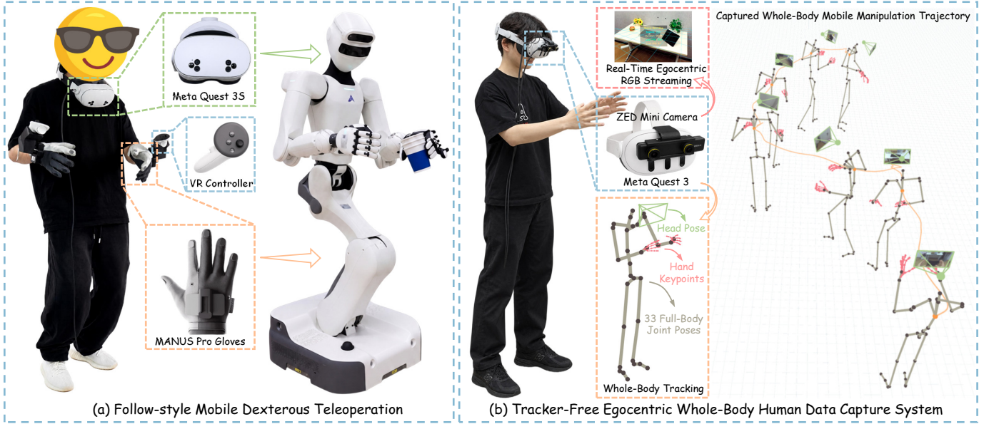
Fig. 2. DexRoam data collection system. (a) Follow-style teleoperation lets one operator drive base, torso, arms, head, and dexterous hands simultaneously via a Meta Quest 3S, VR controllers, and MANUS Pro gloves, with gesture-based episode management. (b) Tracker-free egocentric capture uses a Meta Quest 3 and a head-mounted ZED Mini to record 6-DoF head pose, 33 body joints, 25 joints per hand, and timestamped egocentric stereo RGB, with no external cameras, marker or trackers. Real-time in-headset video streaming keeps the demonstrator’s view identical to the policy observation.
